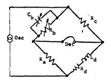
BALANCE EQUATION:  $L_d = R_a R_c C_b$   $R_d = R_a R_c / R_b$ Usually  $R_a = R_c = R_s$ so that:  $L_d = R^2 C_b$  $R_d = R^2 / R_b$
